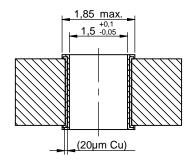
Drill hole specification for chemical surfaces (Ni/Au)
