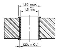
Drill hole specification for chemical surfaces (Ni/Au)
