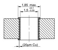
Drill hole specification for chemical surfaces (Ni/Au)
