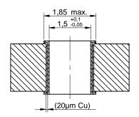
Drill hole specification for chemical surfaces (Ni/Au)
