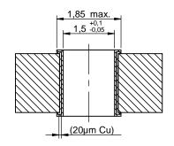
Drill hole specification for chemical surfaces (Ni/Au)
