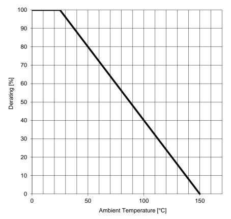
**Steady State Power Dissipation Derating:**
