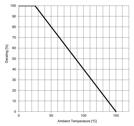
**Steady State Power Dissipation Derating:**
