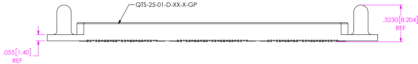
FIG 6 -GP: GUIDE POST SHOWN (QTS-048-01-XXX-D-DP-GP SHOWN) (DIFFERENT AS SHOWN, OTHERWISE SAME AS FIG 1) (AVAILABLE ON STYLE -01 ONLY)
