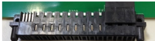
Figure 23 - Mating connector with input exiting flying leads
