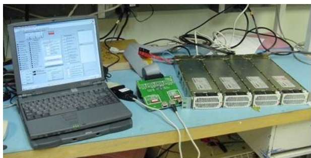
Figure 10 -Test setup using a ABB J85480 shelf
