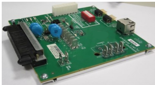
Figure 3 - Single Module CPL interface card for DC-DC converters
