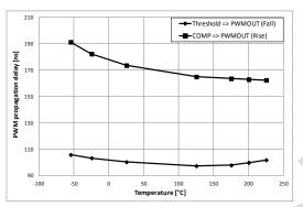
Figure 17. PWM Propagation
