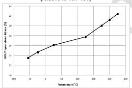
Figure 11: DOUT open drain Ron (VIN=15V)
