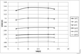
Figure 3: Voltage regulator line regulation (lout =3 mA)
