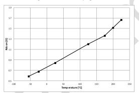
Figure 19: Switching transistor Ron
