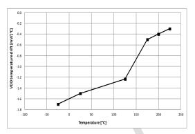
Figure 2: Voltage regulator temperature drift (VIN=15V, lout = 15mA)
