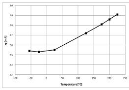
Figure 28. Average current VIN (Primary and both Secondary's in fault; VIN=15V)
