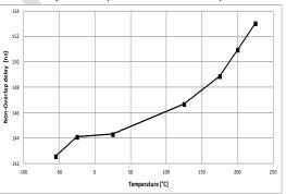
Figure 12: Non-Overlap delay (no external capacitor)
