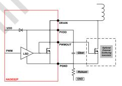
Figure 40. DC-DC output stage
