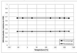
Figure 9: DIN Hysteresis thresholds (relative to VIN=15V)
