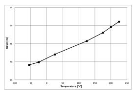
Figure 7: DIN => TX Propagation Delay (modulated interface)
