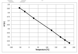
Figure 21: AUX diode Vf (If=1mA)
