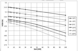
Figure 4: Voltage regulator load regulation (Vin=15V)
