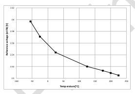
Figure 5: Voltage reference @ FB pin (including OPA offset)
