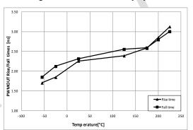
Figure 18. PWMOUT Rise/Fall times (No external load)
