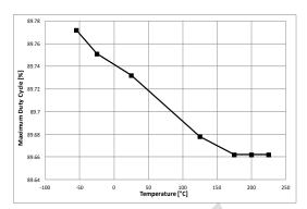
Figure 16: DC-DC Clock Duty Cycle
