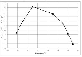
Figure 14: TX oscillator modulationfrequency
