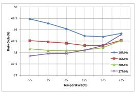
Figure 5: Duty cycle (V<sub>DD</sub>=5V)
