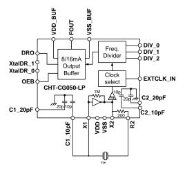
Figure 9. Minimal configuration.
