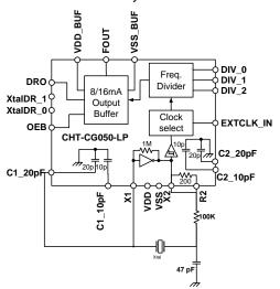
Figure 7. Configuration for 32KHz operation
