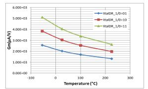
Figure 6: Crystal driver transconductance ( $V_{DD}$ =5V)
