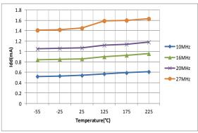
**Figure 2:** Current consumption (V<sub>DD</sub> = 3.3V, OEB = LOW, C<sub>L</sub> = 0pF, XTALDR\_0=1, XTALDR\_1=0)
