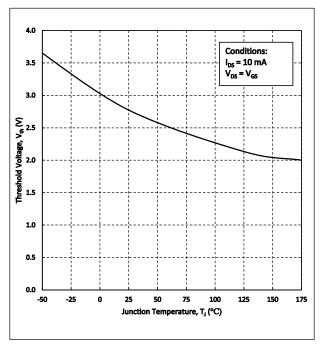
Figure 12. Threshold Voltage vs. Temperature
