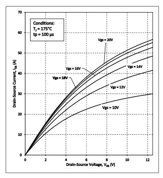
Figure 4. Output Characteristics  $T_J = 175$ °C
