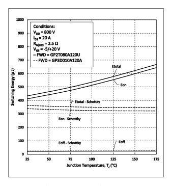
Figure 22. Clamped Inductive Switching Energy vs.
