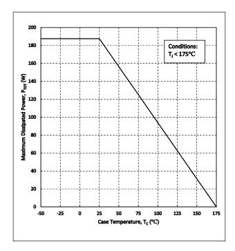
Figure 17. Maximum Power Dissipation Derating vs Case Temperature
