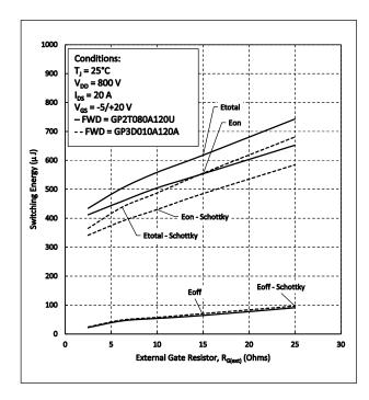
Figure 21. Clamped Inductive Switching Energy vs.  $R_{\text{G(ext)}}$
