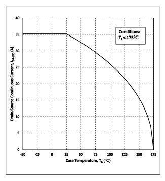
Figure 16. Continuous Drain Current Derating vs.
