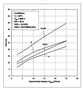
Figure 23. Switching Times vs  $R_{G(ext)}$
