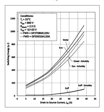
Figure 20. Clamped Inductive Switching Energy vs.
