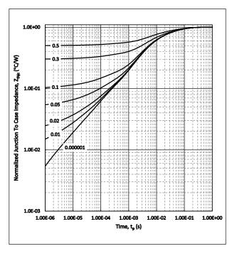
Figure 18. Transient Thermal impedance (Junction to Case)
