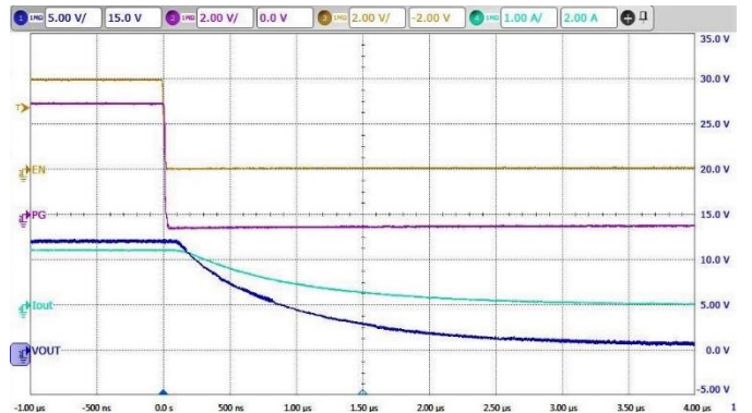
Turn Off Response V_{IN} = 12V, V_{CC} = 5V, V_{EN} = 0V \text{ to } 5V, R_L = 10\Omega
