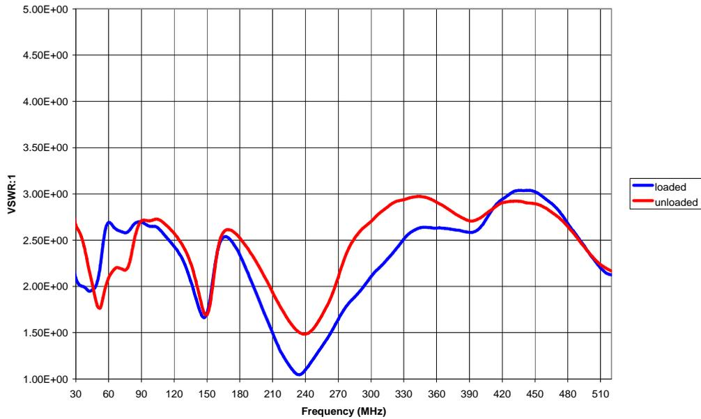
**Figure 1: Typical VSWR with Antenna mounted on a transceiver, 1m above ground.**
