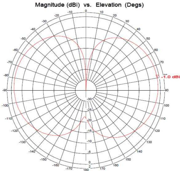
**Figure 3: Typical Elevation Pattern Data @ 75MHz**
