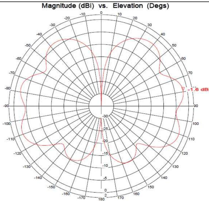
**Figure 7: Typical Elevation Pattern Data @ 400MHz**
