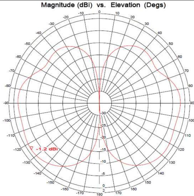
**Figure 6: Typical Elevation Pattern Data @ 300MHz**
