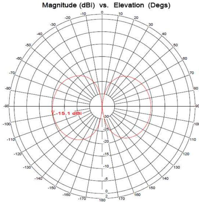
**Figure 2: Typical Elevation Pattern Data @ 45MHz**
