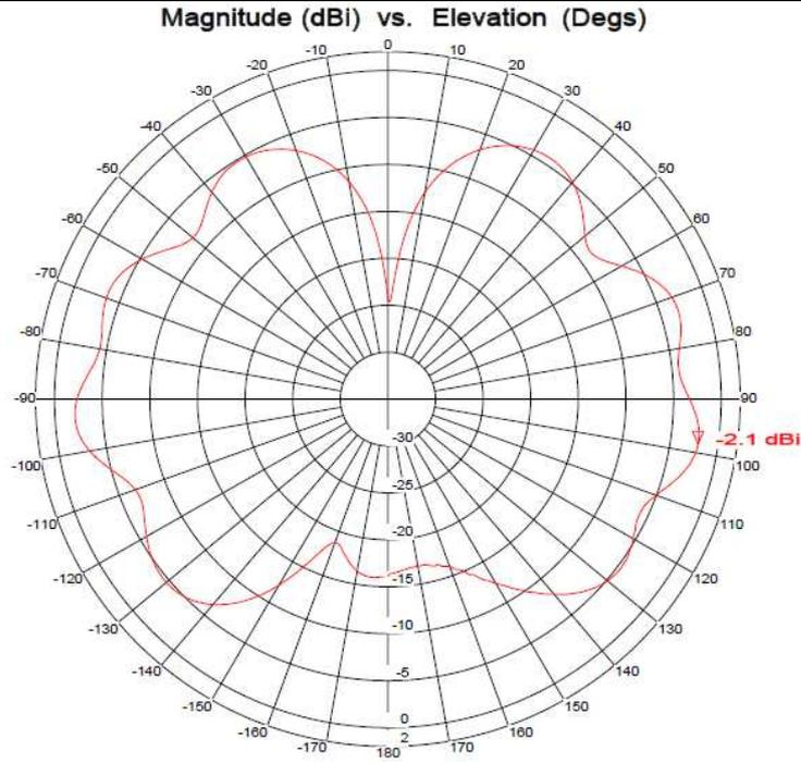
**Figure 8: Typical Elevation Pattern Data @ 500MHz**
